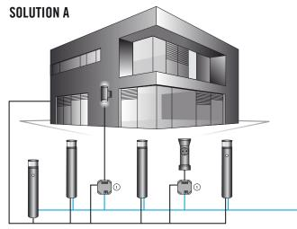
① The DALI actuator (item no. EP10427473/ EP10427480) switches on the "master" light if movement is detected in the field of detection.
