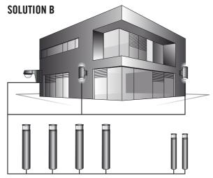
DEFENSOR motion detectors are ideal for controlling ALVA lighting for 230 V. This creates a visually harmonious lighting solution while the safety and control functions of the DEFENSOR series increase building safety even further.
