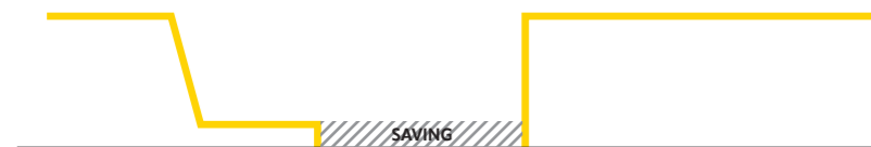
Energy consumption with power cut-off: DALI drivers do not consume power in stand-by mode
