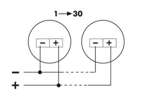
9 V battery operation Note: Interconnection with max. 30 detectors, max. line length 300 m.
